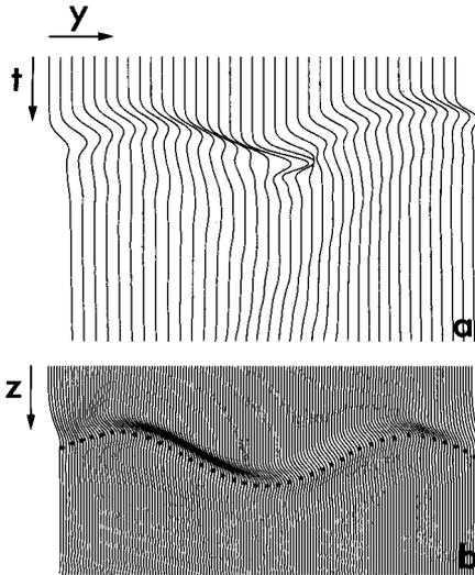
Fig. 4. Migration of a synthetic time section (a) corresponding to a sinusoidal reflector in a variable velocity medium. The peak of the migrated image in the  $y$ - $z$  plane (b) coincides with the correct solution, which is shown as the dotted line. (See caption to fig. 1.)
