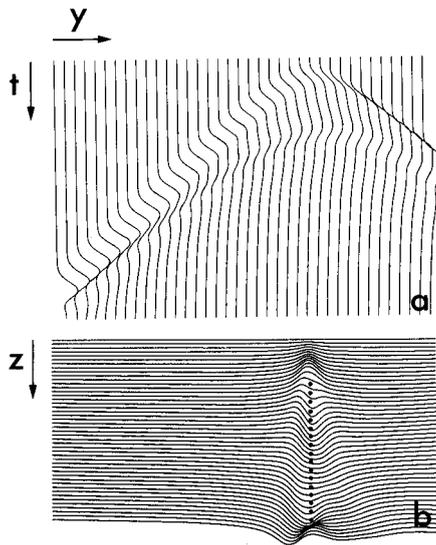
Fig. 3. Migration of a synthetic time section (a) corresponding to a vertical reflector. The peak of the migrated image in the  $y$ - $z$  plane (b) coincides with the correct solution, which is shown as the dotted line. (See caption to fig. 1.)
