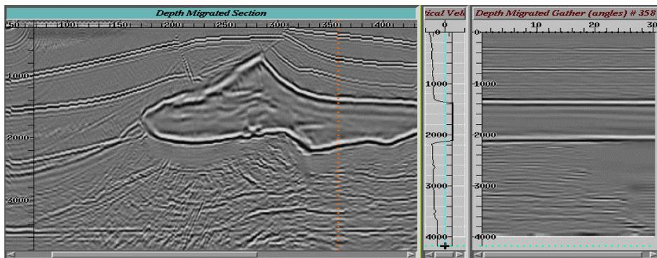
Figure 3: Result of 3-D depth imaging from the 3-D SEG-EAGE salt model, inline 360, with an example of an angle domain CIG.
