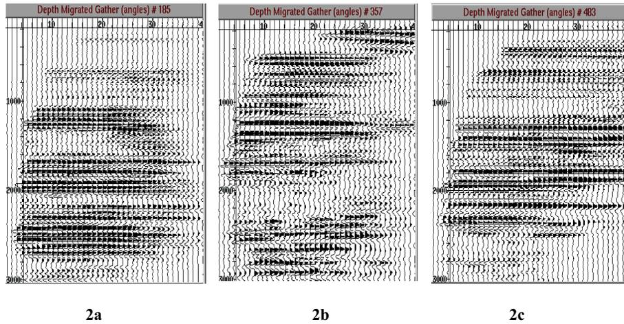
Figure 2: Example of common reflection angle gathers used to create the depth image above (figure 1) in three different locations: a) CIG 185, b) CIG 357 and c) CIG 483. Note, that although CIG-357 is located at the complex area, the migrated events are relatively continues for large range of reflection angles (up to 40 deg.).
