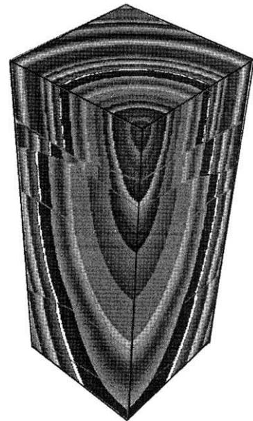
Figure 4: Vertical slice of the cube shown in figure 3. The traveltime field consists of body waves only.
