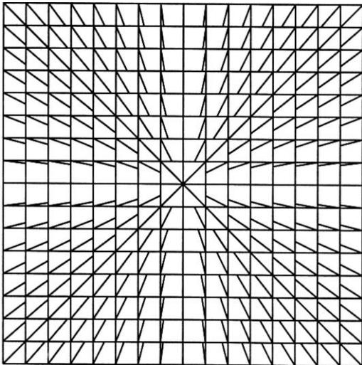
Figure 1: Mixed grid. Horizontal slice through the 3D mesh for a case of circular wave-fronts. In the solution scheme, downward extrapolation is done on the cartesian nodes, and head-wave to body-wave corrections are made on the cylindrical nodes.
