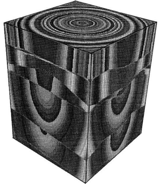
Figure 3: Traveltime cube calculated for the salt mode/presented in figure 2. The cube size is 200x200x300.
